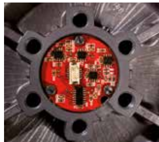
OFBS The Optical Feedback System (OFBS) enables built-in monitoring of LED degradation over time.
