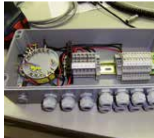
LT Control Unit LEDFlasher is the controller in the control unit. Each unit can control max 10 light tubes.
