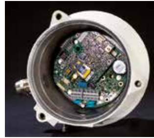
Light Guard GSM GSM unit and antenna integrated in the lantern for remote monitoring and control.
