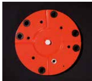
Installation The bottom plate supports installation on structure with 3 x M12 bolts on a 200 mm diameter. The mounting holes are galvanic isolated with plastic isolators. PTFE breathing vent for pressure release.
