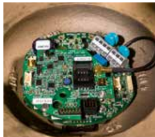
GSM GSM unit and antenna integrated in the lantern for remote monitoring and control. For more information please see the LightGuard Section.
