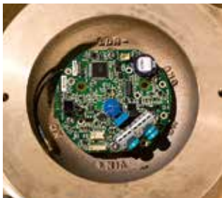
GPS GPS unit and antenna integrated in the lantern for wireless synchronization and for position monitoring. The integrated GPS antenna is moulded and survives ice pressure.
